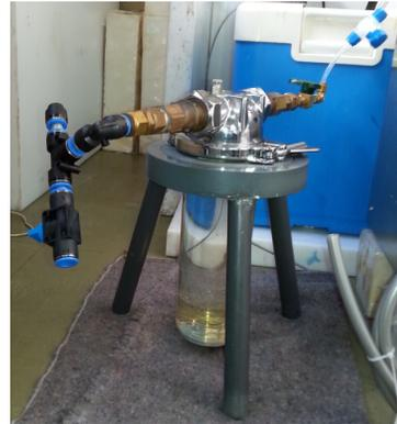
**Fig. 2.** Chamber on a tripod, with all the connections of the cap assembled. The yellow tonality observed, especially in lower part of the chamber's body, is due to the gel covering the chamber walls and bottom.
