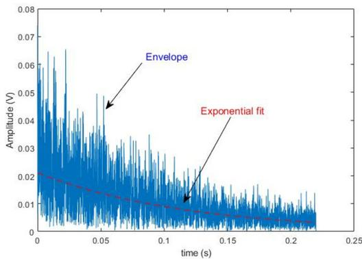
**Fig. 6.** Best fit of the exponential in Eq. 6 to the amplitude envelope of the pulse shown in Fig.5.
