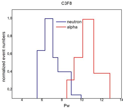
**Fig. 7.** Histogram presenting the calibrations made using alpha-particle and neutron sources.
