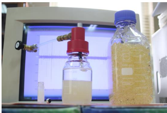
Figure 1. The evaluated C 2 ClF 5 devices. From left to right: 4 mL SDD and microphone; 150 mL SDD with a modified cap to embed the signal and pressure feedthroughs (note the microphone embed in a glycerin layer covering the translucent emulsion); 1 L SDD displaying gel fractures after exposure to high fast neutron fluence.
