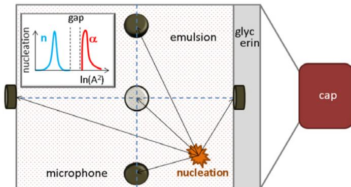
**Figure 1.** Schematic view of the SDD (in horizontal position) with a 5-microphone arrangement for the spatial localisation of the nucleations. The inset graph represents the amplitude ( $A$ ) histograms of the acoustic signals corresponding to nucleations induced by recoiling nuclei following neutron interactions ( $n$ ) and alpha-induced events ( $\alpha$ ), clearly separated by a gap.
