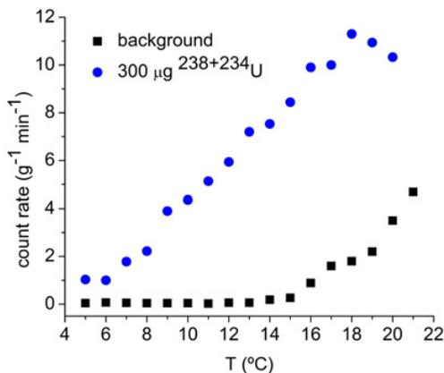
**Figure 2.** Temperature dependence of the response of a 150 ml SIMPLE SDD, doped with a 1mg/ml U solution and undoped (background).
