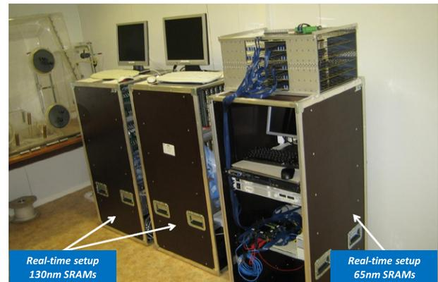
**Fig. 4.** General view of the experimental room dedicated to microelectronics experiments inside the Modane underground laboratory. The two automatic test equipments are dedicated to the real-time SER test of 130 nm and 65 nm SRAM circuits.
