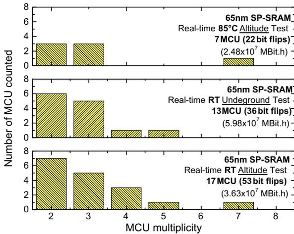
**Fig. 6.** Distribution of the MCU multiplicity (i.e. number of bit flips per MCU event) for the 11 MCU events detected during the altitude test (SP-SRAM). These MCUs involves a total of 38 bit flips which correspond to physical adjacent bit cells (in the memory plan) in all cases.
