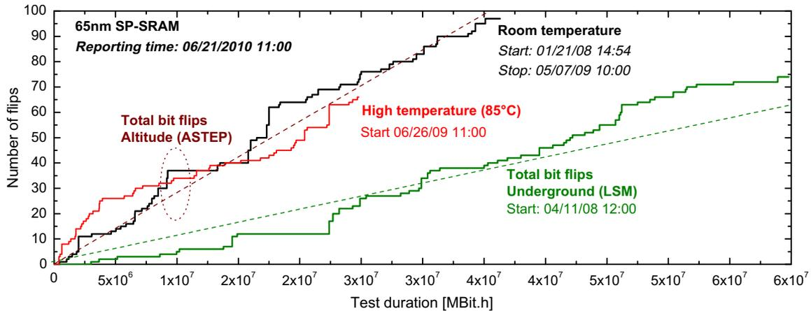
**Fig. 5.** Cumulative total fails (i.e. total bit flips) versus test duration for the 65 nm SP-SRAM during both altitude and underground experiments. Test has been conducted under nominal conditions:  $V_{DD} = 1.2$  V, standard checkerboard test pattern and room temperature (except for the high temperature test conducted at 85 °C using a heating oven).
