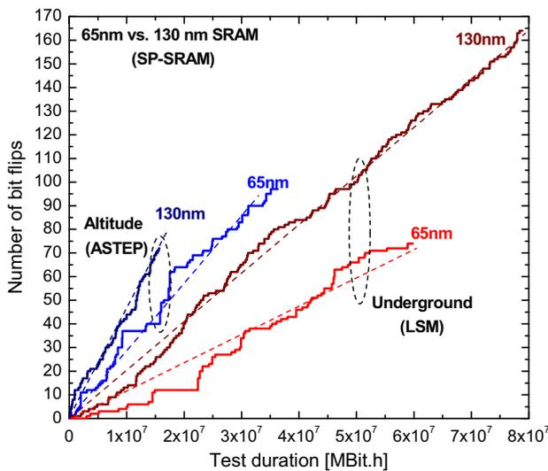
**Fig. 7.** Cumulative total fails versus test duration for both 130 nm and 65 nm SP-SRAMs detected in altitude and underground. Test has been conducted under nominal conditions for both technologies:  $V_{DD} = 1.2$  V, room temperature, standard checkerboard test pattern. For 130 nm data, experiment periods are [March 31, 2006–November 6, 2006] for the altitude test and [October 16, 2007–November 24, 2008] for the underground test.
