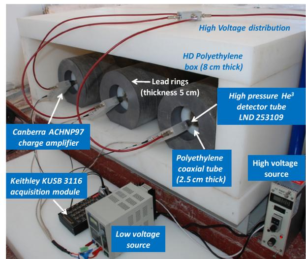
**Fig. 2.** Detailed view of the PdBNM showing the extremities of the cylindrical neutron detector tubes connected to the charge amplifiers and to the acquisition module (electronic counters).
