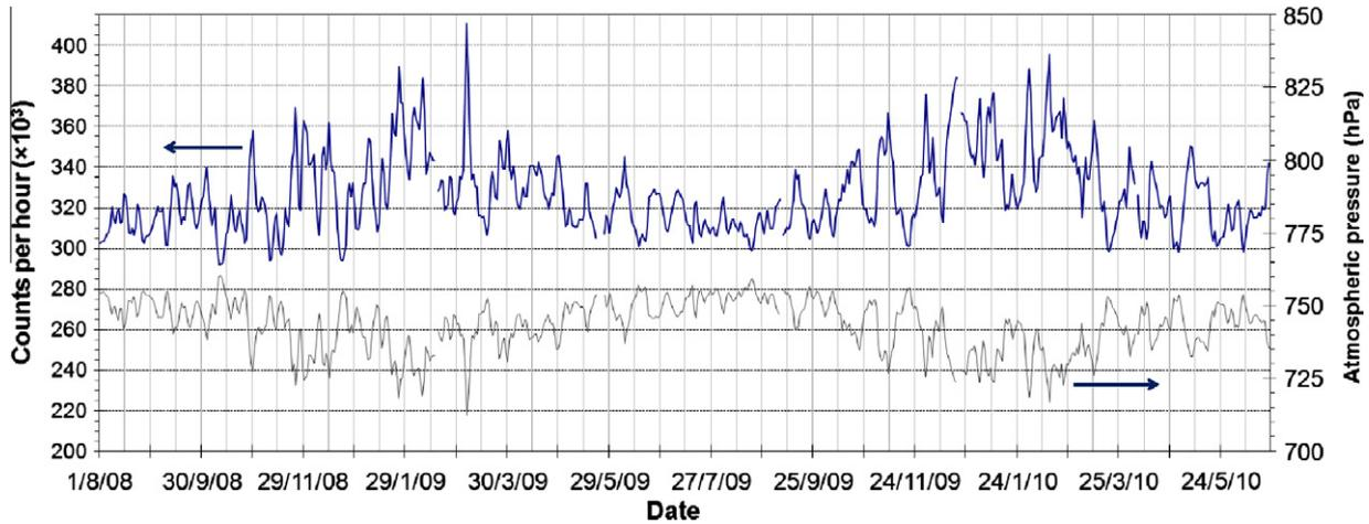
**Fig. 3.** Plateau de Bure neutron monitor response recorded from August 1, 2008 to June 21, 2010. Data are uncorrected from atmospheric pressure and averaged over 1 h.  $\sim 30\%$  variations in neutron flux are evidenced, with two peaks (around  $4 \times 10^5$  counts/h) corresponding to the passage of two severe atmospheric depressions (the first peak correspond to the Klaus storm on January 25, 2009).
