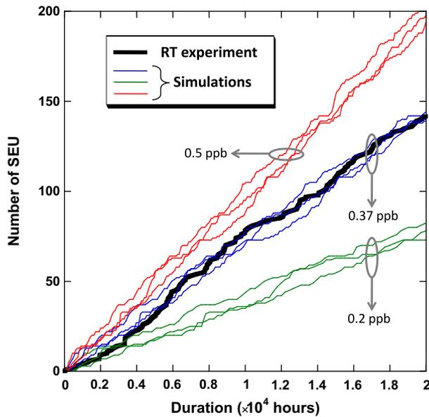
Fig. 10. Cumulative number of SEU versus test duration for the underground SER experiment (bold line). Several error distributions (thin lines) computed by Monte-Carlo simulations for different contaminations levels (0.2, 0.37 and 0.5 ppb of  $^{238}\text{U}$ ) are superimposed.
