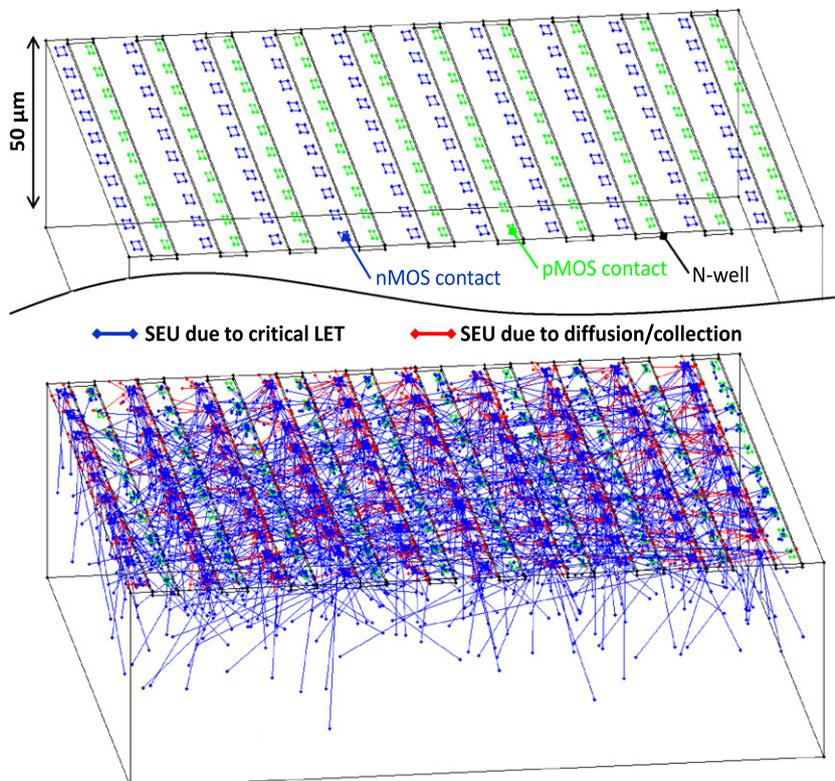
**Fig. 9.** Layout (up) and simulation result (down) of a  $10 \times 10$  SRAM block. Blue segments (respectively red) represent alpha-particle tracks given a SEU due to critical LET (respectively due to diffusion–collection). In this example, a total of 100,000 alpha-particles have been generated for each nuclei of the decay chain. (For interpretation of the references to colour in this figure legend, the reader is referred to the web version of this article.)
