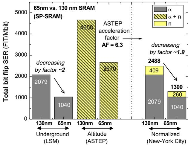
**Fig. 8.** Synthesis of experimental real-time SER values obtained for both 130 nm and 65 nm SP-SRAM from altitude and underground experiments and normalization of the SER at the reference flux of New-York City (sea-level) [18] taking into account: (i) the alpha contribution for the altitude test (fixed to the value measured at LSM) and (ii) the ASTEP acceleration factor  $AF = 6.3$  for the neutron flux in altitude (experimentally measured using the Plateau de Bure neutron monitor).
