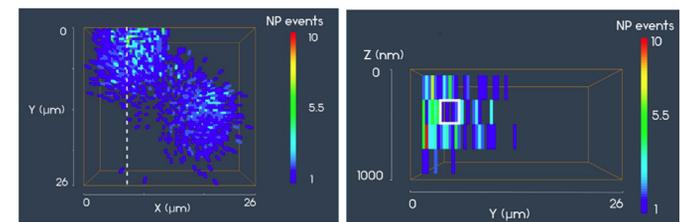
MORIA 3D model of the distribution of Cu and the depth distribution of Cu along the white line, from [1].
