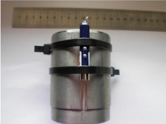
Figure 4. Lateral view of irradiator with a mini-laser tied to it
