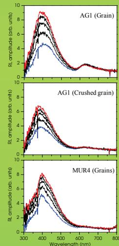
RL spectra, repeated irradiation with 20 kV X-ray source
