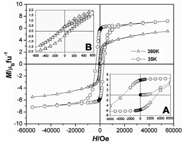
Fig. 5. Field dependence of the magnetization and hysteresis loops for the  $UFe_5Ga_7$  compound. Insets: Details of the  $M(H)$  curves at 35 K (A) and 280 K (B).
