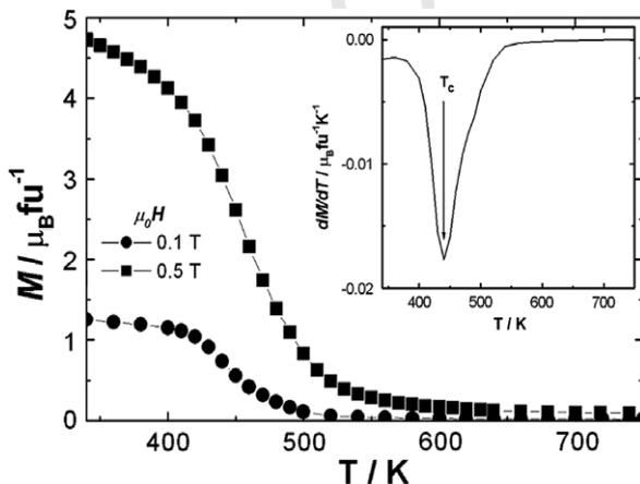
Fig. 4. High temperature dependence of the magnetization for the  $UFe_5Ga_7$  compound. Inset shows in detail the temperature derivative of the magnetization.
