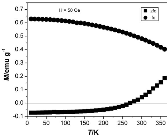
Fig. 3. Low temperature dependence of the magnetization for the  $UFe_5Ga_7$  compound.
