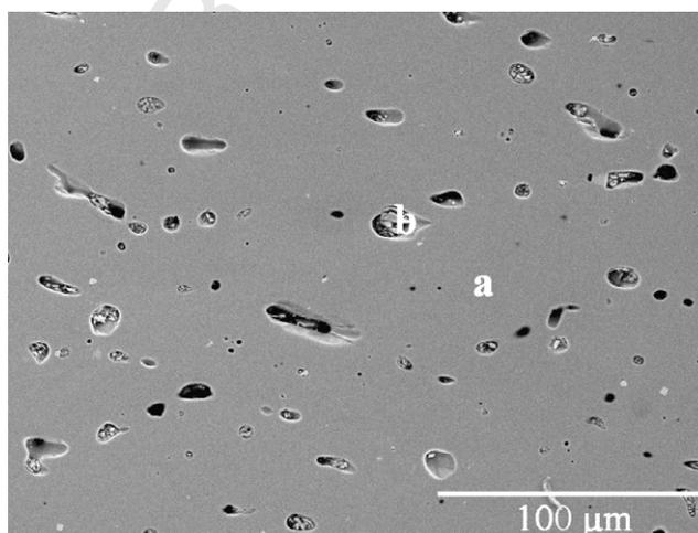
Fig. 2. SEM micrograph of the sample  $\text{UFe}_5\text{Ga}_7$ : (a)  $\text{UFe}_7\text{Ga}_5$ , (b) eutectic phase.
