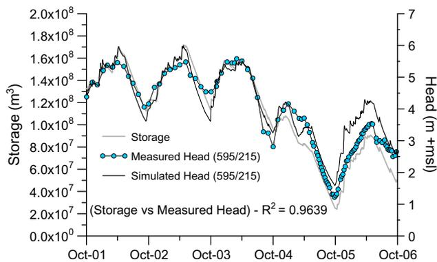
Fig. 3. Observed and simulated hydraulic head at piezometer 595/215 and simulated storage of the QS.
