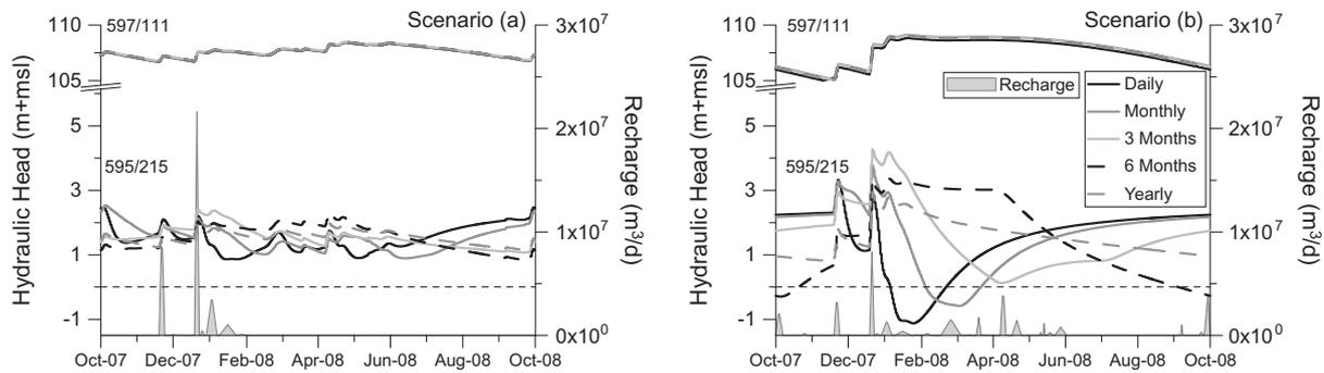
**Fig. 4.** Variation of hydraulic head at piezometers 595/215 and 597/111 for the hypothetical abstraction rates considering current temporal distribution of recharge (scenario a, left) and considering predicted temporal distribution of recharge (scenario b, right); for location of the piezometers see Fig. 1.
