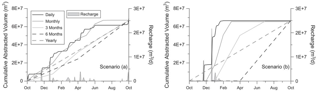
Fig. 5. Cumulative abstracted volumes per cyclical year of the considered time scales for scenario a (left) and scenario b (right).
