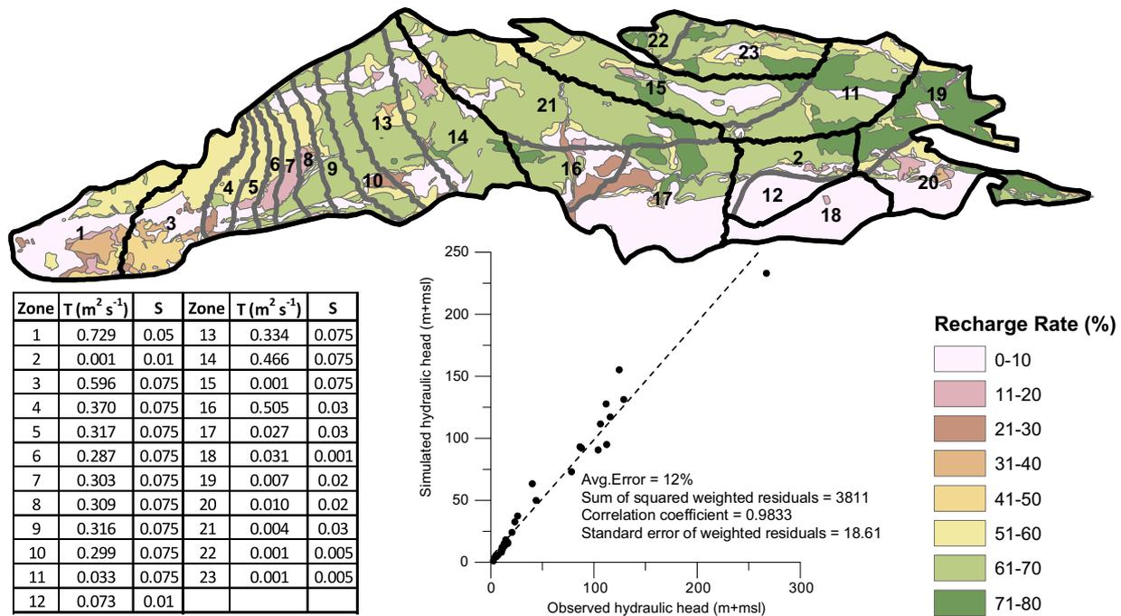
Fig. 2. Map of chosen transmissivity zones (grey lines) and storage coefficient zones (black lines) as well as spatial distribution of recharge ratio (top), optimised values obtained by calibration (bottom left) and resulting plot of modelled versus observed hydraulic heads (bottom right).
