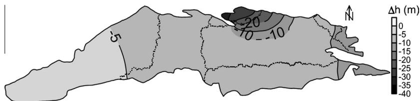
**Fig. 8.** Difference between simulated hydraulic heads at the end of September 2009 with maximum abstraction rates based on a monthly time scale and simulated heads in the same period with measured abstraction rates.
