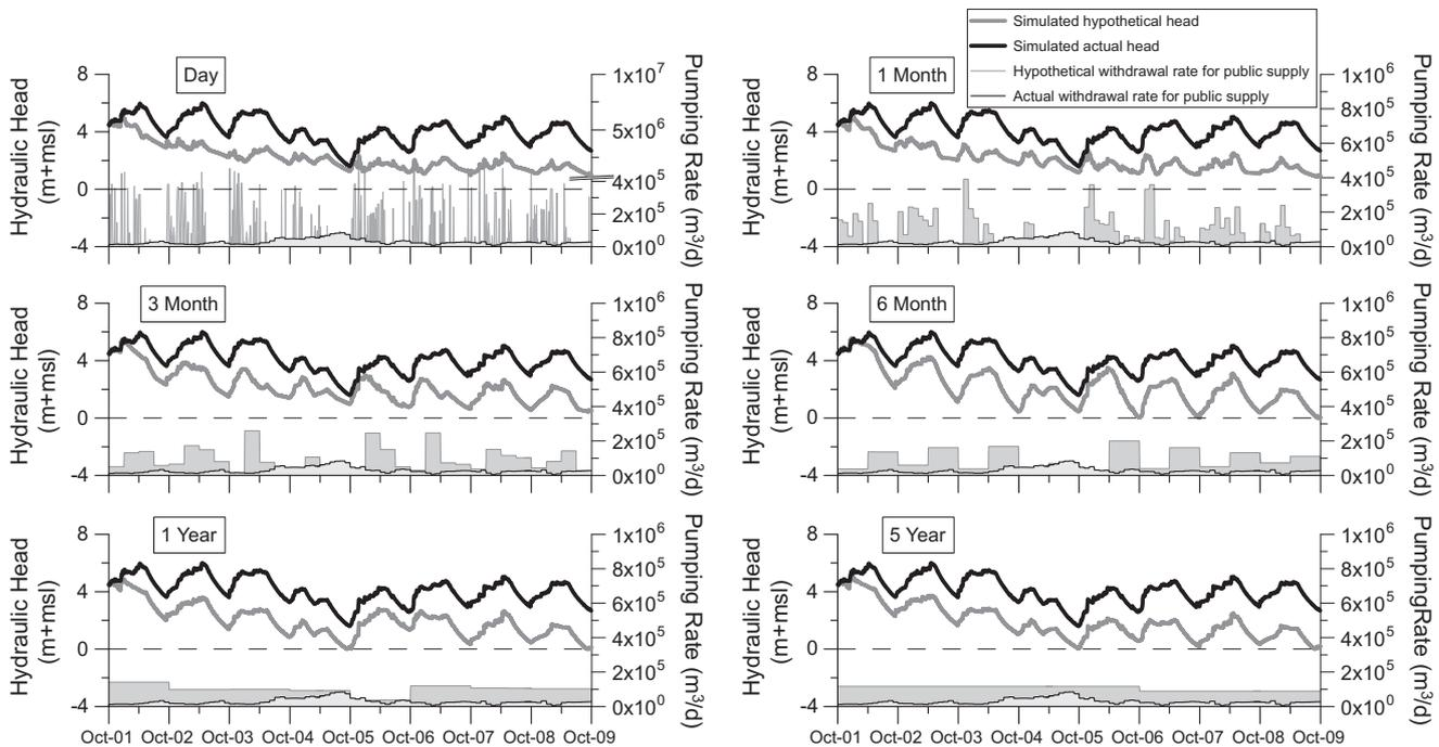
Fig. 7. Variation of hydraulic head at piezometer 595/215 for the considered hypothetical maximum abstraction scenarios; extractions for irrigation during spring and summer months are considered in the model, but not represented here.
