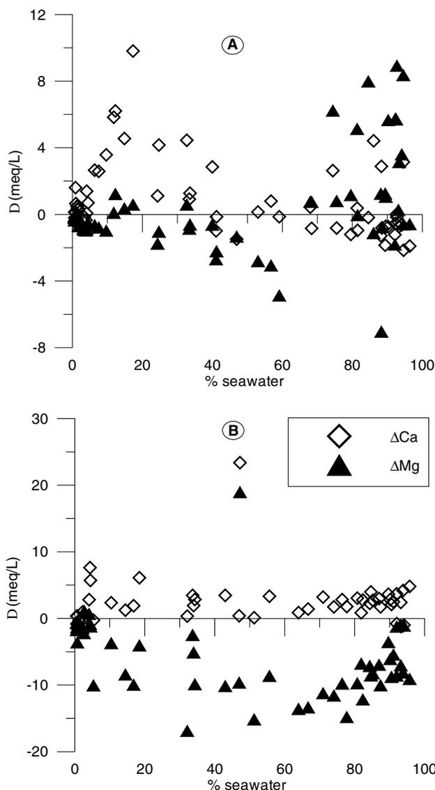
Fig. 8.  $\Delta\text{Ca}^{2+}$  and  $\Delta\text{Mg}^{2+}$ -% seawater plots for the samples taken in July 1998 (A) and November 1998 (B).
