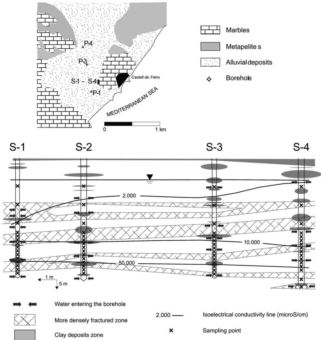
Fig. 2. Location and cross-section of sampling wells with log interpretations for the 4 monitoring wells tapping the marbles. S1 is nearest the sea.
