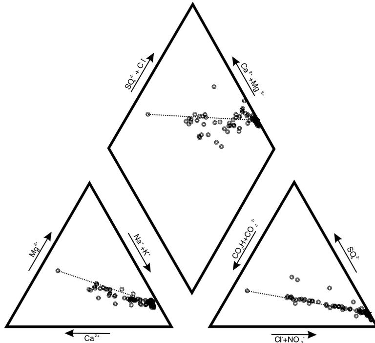
Fig. 3. Piper diagram, showing theoretical freshwater–seawater mixing line.
