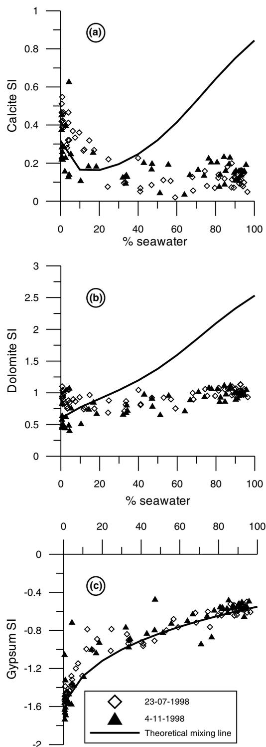
Fig. 6. Calcite (a), dolomite (b) and gypsum (c) saturation indices for the samples taken in July 1998 and November 1998. The theoretical saturation indices for conservative mixing between freshwater and seawater is also shown.
