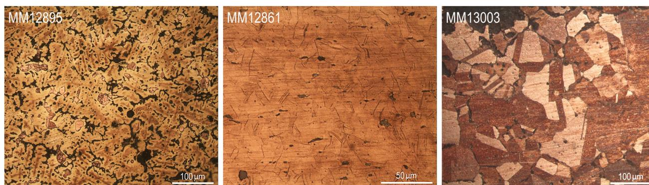
**Fig. 2** Optical microscopy images of fibulae MM12895 and MM12861 and finger ring MM13003 (bright field, etched: *pink* inclusions in MM12895 are redeposited copper, and *dark* inclusions in MM12861 are copper oxides)
