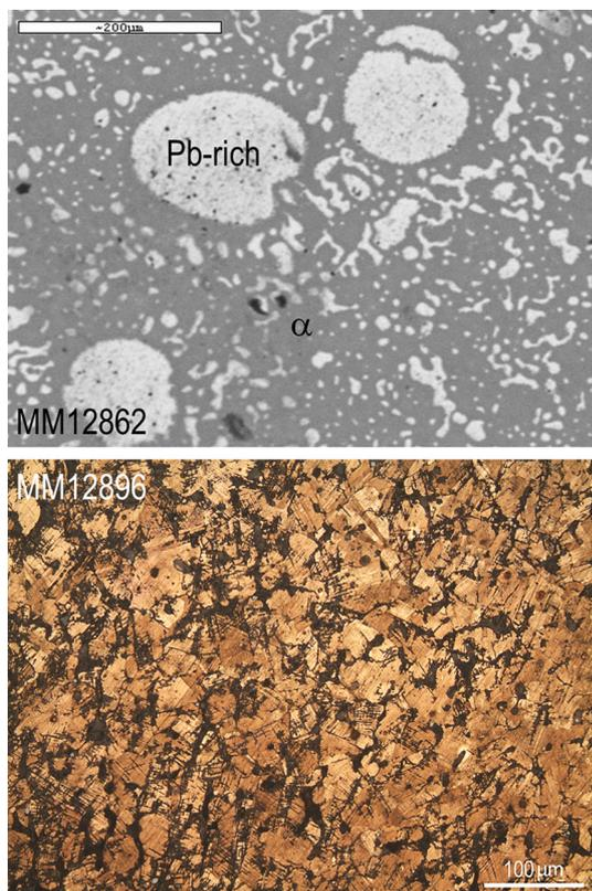
**Fig. 3** SEM–BSE image of jug handle MM12862 (SEM–EDS results show 4.9 wt% *Sn* and 21.4 wt% *Pb*, and the small difference in micro-EDXRF results are related with the heterogeneous distribution of lead-rich inclusions in copper–tin  $\alpha$  phase) and optical microscopy image of snaffle bit MM12896 (bright field, etched)
