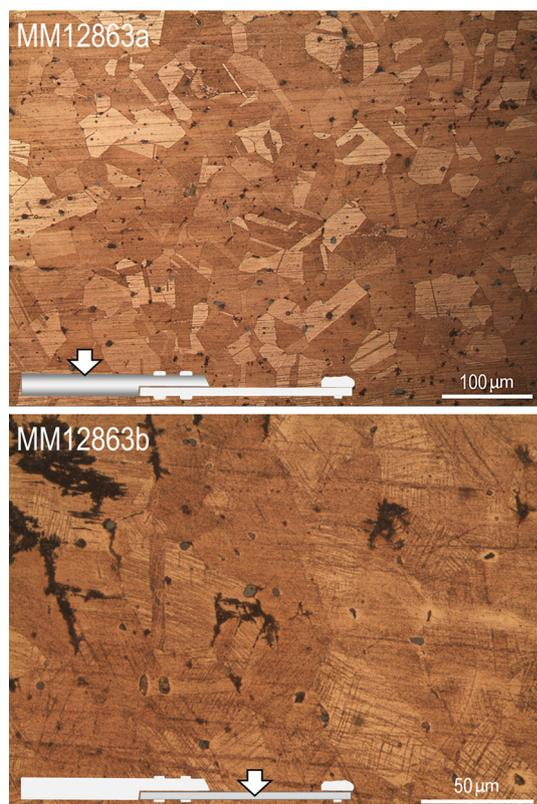
**Fig. 5** Microstructures of segments from handle MM12863 (bright field, etched; *bottom left* observed sections of rod)
