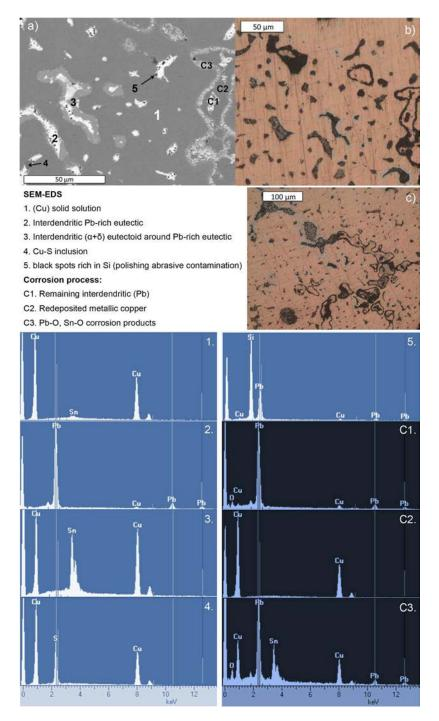
Figure 6. Microstructure of anthropomorphic handle attachment MA020: a) SEM image with several points of analysis by EDS related to original microstructure (1-5) and corrosion process (C1-C3); b) OM image of the area analysed by SEM (BF); c) OM general view (BF).
