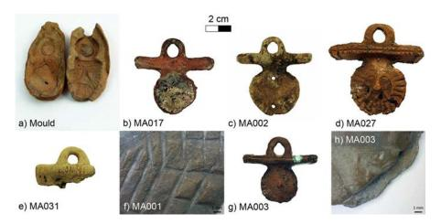
Figure 2. a) Bivalve clay mould for the production of anthropomorphic handle attachment of type III found in *Conimbriga*; b) MA017 with remnants of solder at the back; c) MA002 with two rivet holes; d) Casting defects of MA027 with several macropores (black colour); e) MA031 broken artefact with visible cracks; f) Stereo microscope (SM) image of chisel work on MA001; g) MA003 showing wear on ring; h) SM image of MA003 flashing.
