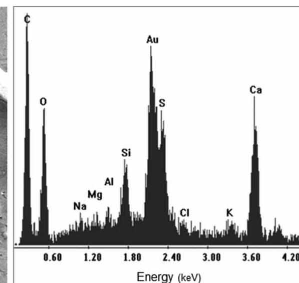
**Figure 4** SEM image of a corroded area in the white glaze and EDX spectrum collected from the area defined by a circle.
