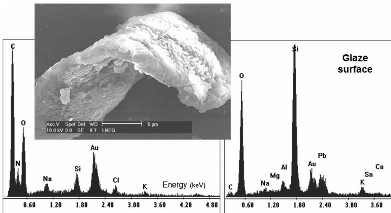
Figure 5 Comparison of EDX spectra collected from a microorganism and from the glaze surface.
