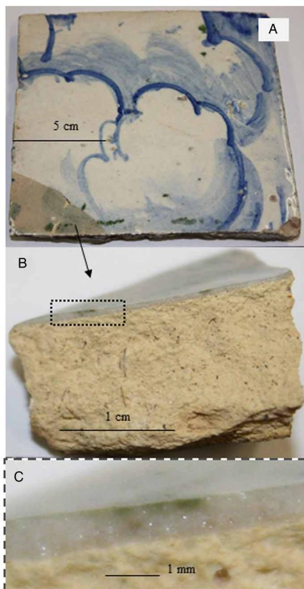
**Figure 1** Studied blue-and-white tile (A) and magnified view of a fragment presenting green stains (B) plus a detail (C) showing that these stains are confined to the glaze surface.
