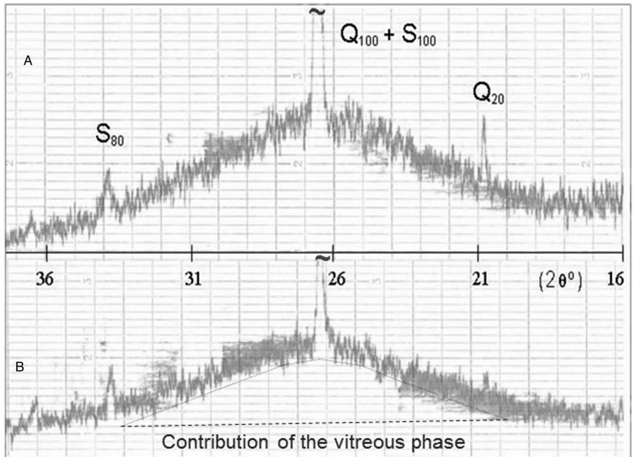
Figure 3 X-ray diffraction patterns obtained for irradiated areas in the studied tile fragment: white glaze (A); green stain (B); the relative intensities of assigned diffraction peaks from quartz (Q) and cassiterite (S) are indicated.
