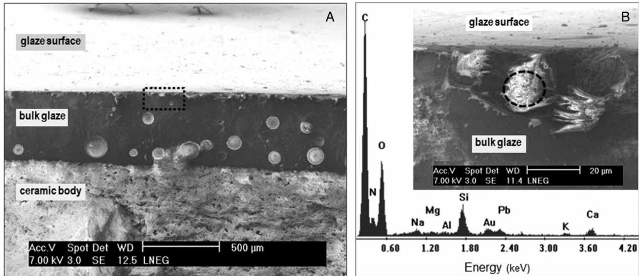
Figure 2 SEM images collected from the fragment reproduced in Fig. 1B: (A) profile view showing vacuoles within the glaze with a rectangle assigning the studied area; (B) detail of this area and EDX spectrum collected from an irradiated green stain (defined by a circle).
