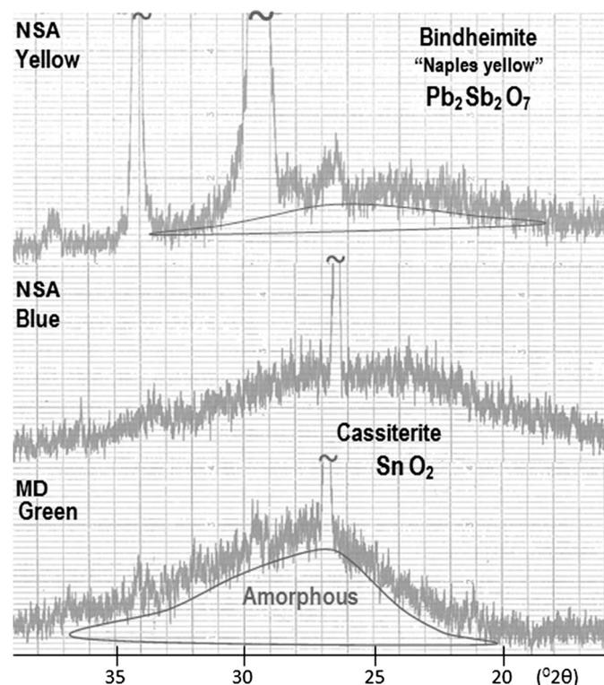
**Fig. 2.** X-ray diffraction (XRD) patterns (Cu Kα radiation) collected from glaze fragments: MD – *Madre de Deus* Church (16th century); NSA – *Nossa Senhora dos Aflitos* Church (17th century).
