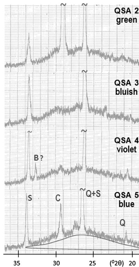
**Fig. 3.** XRD patterns collected from 18th century glaze fragments (QSA – *Quinta de Santo António*). The contribution of an amorphous phase is assigned; identified crystalline phases: S, cassiterite (SnO<sub>2</sub>); Q, quartz (SiO<sub>2</sub>); C, calcite (CaCO<sub>3</sub>); B?, braunite (3Mn<sub>2</sub>O<sub>3</sub>·MnSiO<sub>3</sub>).
