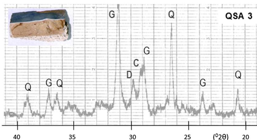
**Fig. 4.** XRD pattern collected from the ceramic body of a QSA tile sample. Assigned phases by decreasing representativity: G, gehlenite ( $\text{CaAl}_2\text{SiO}_7$ ); Q, quartz ( $\text{SiO}_2$ ); D, diopside ( $\text{CaMgSi}_2\text{O}_6$ ); C, calcite ( $\text{CaCO}_3$ ).
