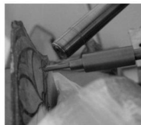
Fig. 2: Photograph during the experiments with the proton beam using the external set-up. Object: Roman glass.
