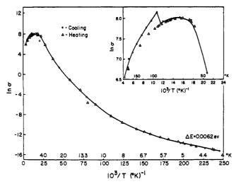
Figure 1. Natural logarithm of  $\sigma$  in ohm<sup>-1</sup> cm<sup>-1</sup> vs.  $10^3/T$  for sample no. JPF-5.  $\Delta E$  is calculated from  $\sigma = \sigma_0 e^{-\Delta E/2kT}$ . Insert shows high-temperature region expanded showing hysteresis between cooling and heating curves at the transition; cooling curve determined first.
