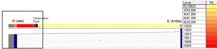
142 143 144 Figure 4 – Vertical section of the aquifer with the simulated chloride concentration in observation point after 1 day of flood; square represents the aquifer zone in Figure 5; dark line is the groundwater level.
