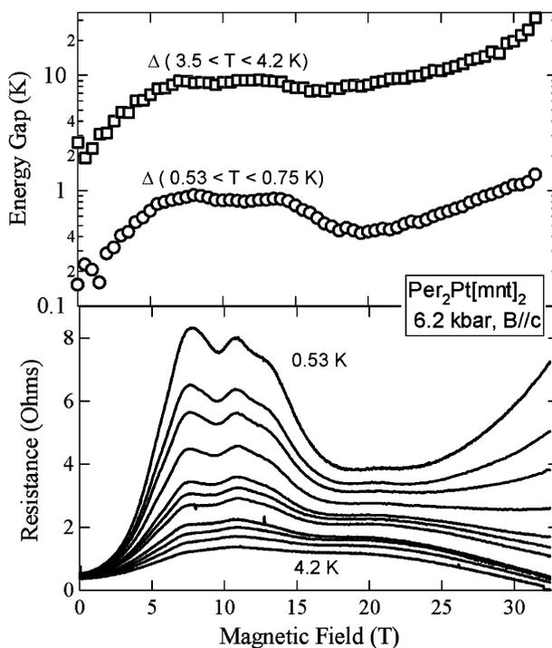
Fig. 10. Lower panel: Magnetoresistance of  $\text{Per}_2\text{Pt}(\text{mnt})_2$  at 9.5 kbar vs. temperature for  $B \parallel c$ . Upper panel: energy gaps at low and high temperatures derived from Arrhenius analysis.
