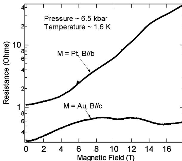
Fig. 9. Magnetoresistance of  $\text{Per}_2\text{Pt}(\text{mnt})_2$  and  $\text{Per}_2\text{Au}(\text{mnt})_2$  at 6.5 kbar at low temperatures.
