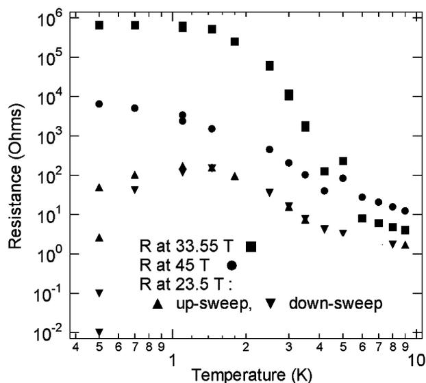
Fig. 4. Temperature dependent resistance for  $\text{Per}_2\text{Pt}(\text{mnt})_2$  in the FICDW region. Arrhenius analysis was performed in the 2–4 K range of the data. At 23.5 T, the sample becomes metallic below 1.8 K. The scatter in the 0.5 K data for 23.5 T is from measurements from different sweeps through this region (see text for discussion).
