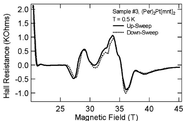
Fig. 8. Hall effect in the FICDW state based on subtraction of field forward and field reversed signals ( $B \parallel c$ ) by sample rotation through  $180^\circ$  for two field sweeps up and two field sweeps down. Finite Hall signals in the FICDW state have been observed in a total of four samples in preliminary studies, but it should be noted that the details vary from sample to sample.
