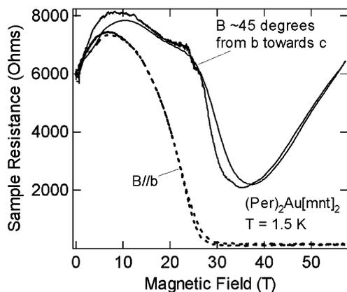
Fig. 3. Pulsed field measurements on  $\text{Per}_2\text{Au}(\text{mnt})_2$  for two orientations at 1.5 K.
