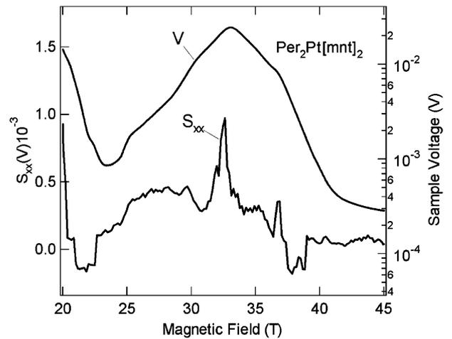
Fig. 7. Simultaneous thermopower and resistance measurements of  $\text{Per}_2\text{Pt}(\text{mnt})_2$  in the region of the FICDW phase.
