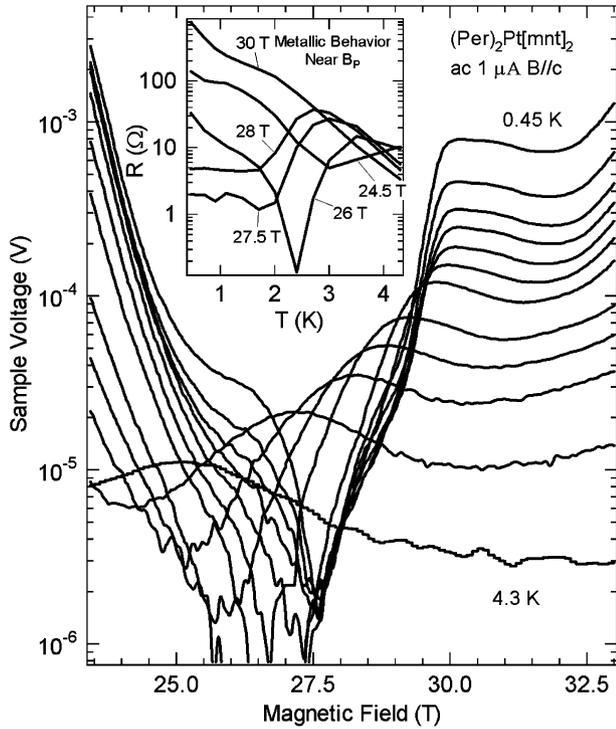
Fig. 5. Field and temperature dependence of the resistance of  $\text{Per}_2\text{Pt}(\text{mnt})_2$  for  $B \parallel c$  in the vicinity of  $B_p$  for a second sample. In the range  $24 < B < 30$  T the resistance shows metallic behavior over a range of temperature and field. dc  $I$ - $V$  curves in the vicinity of  $B_p$  show Ohmic behavior.
