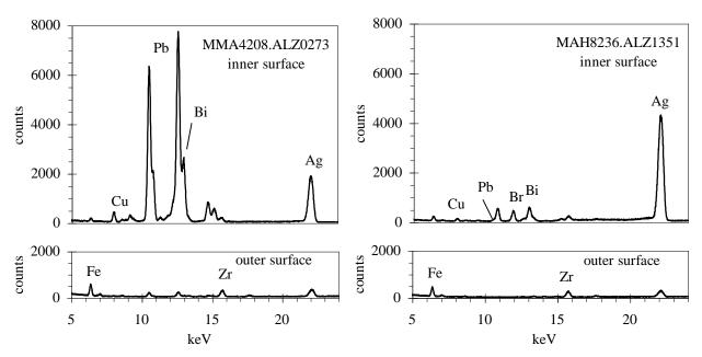
Fig. 7 - EDXRF analysis of the inner and outer surfaces of two crucibles fragments from Almaraz.
