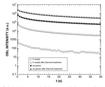
**Fig. 3.** Synthetic quartz crystals, both as-grown and hydrogen swept, "Premium Quality"(Sawyer Research Products, Eastlake, Ohio). Al content was around 10 ppm; the concentrations of alkali ions were approximately 1–3 ppm and 0.1 ppm in the asgrown and H-swept respectively. Samples were cut in the form of discs, 10 mm diameter and 1 mm thickness. (Dose: 50 Gy measured at 125 °C with preheating 10 s at 220 °C). Thermal treatment consists of 16 h at 1000 °C.
