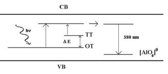
Fig. 4. Schematic diagram of the proposed model. TT Thermal Trap, OT Optical Trap.
