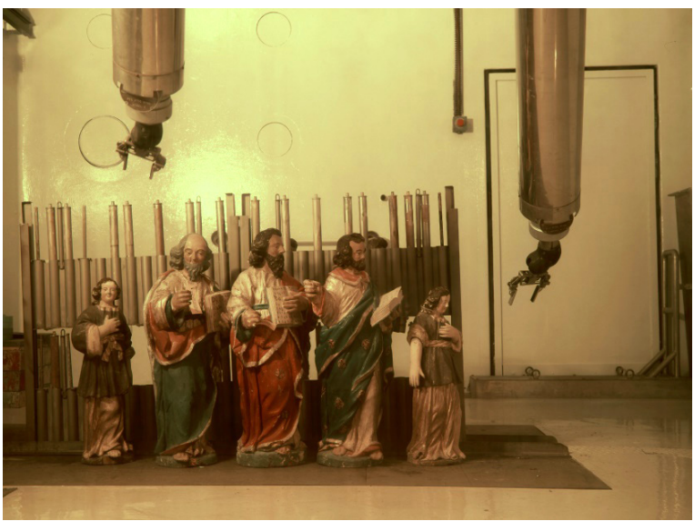
FIG. 26.2. Irradiation of polychrome statues for insect eradication.
