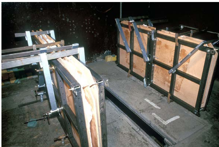
FIG. 17.4. Impregnated parquet panels maintained in steel frames inside the irradiation chamber.
