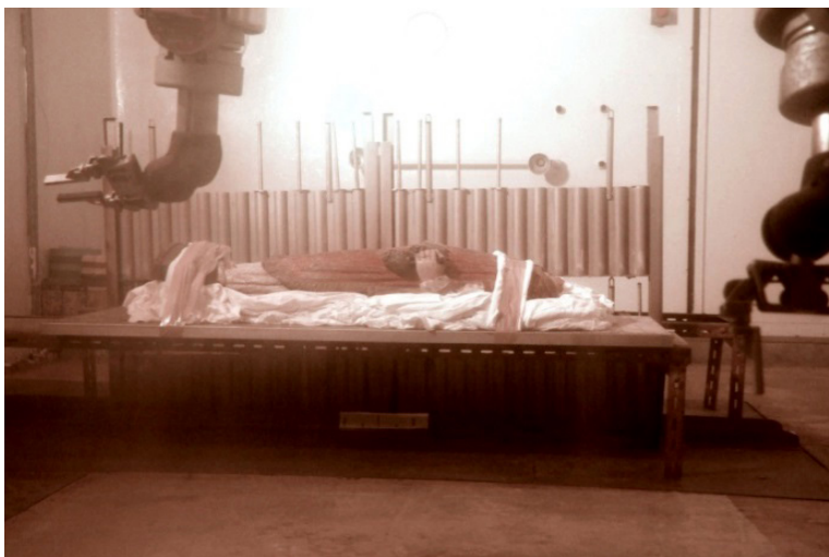
FIG. 16.4. The impregnated sculpture in front of the gamma ray source for the in situ solidification of the resin.
