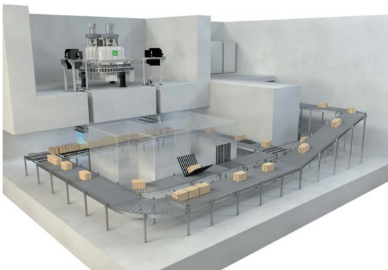
FIG. 6.2. Layout of a typical EB irradiation facility (courtesy of IBA, Belgium).
