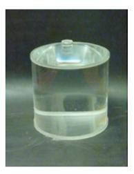
**Figure 1.** The phantom for the calibration of eye lens dosemeters proposed by the ORAMED project.
