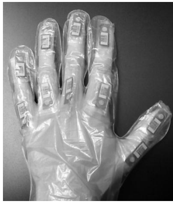
FIG. 1. Dominant hand with ten extremity doseimeters placed at the tip and base of each finger
