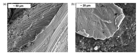
**Figure 8.** SEM SE images of the gilded regions of the silver-based triangular head brooches: (a) fire-gilding with a gold-mercury mixture; (b) fire-gilding with a gold foil (source: M.F. Guerra, C2RMF).
