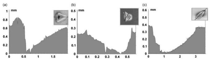
**Figure 4.** Extracted profiles for a triangle produced on a silver plaque by: (a) engraving (with the 'volcanic' type border due to metal removal); (b) stamping (with slight deformation peak on the border); (c) chasing (regular valley without borders).
