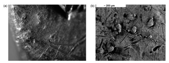
**Figure 3.** PGE inclusions on the bezel of a Hellenistic finger ring: (a) binocular image; (b) SEM SE image (source: M.F. Guerra, C2RMF).
