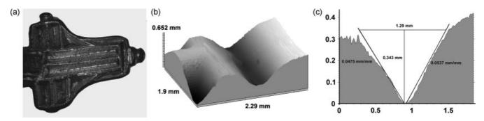
**Figure 9.** Silver-based triangular head brooches: (a) the head region analysed by micro-topography; (b) 3D representation in syntheses of data collected by micro-topography with an optical sensor with a measurement field of 3000  $\mu$ m for an acquisition frequency of 100 Hz and a quantisation step of 5  $\mu$ m × 50  $\mu$ m; (c) extracted profile showing the form and dimensions of the tool.
