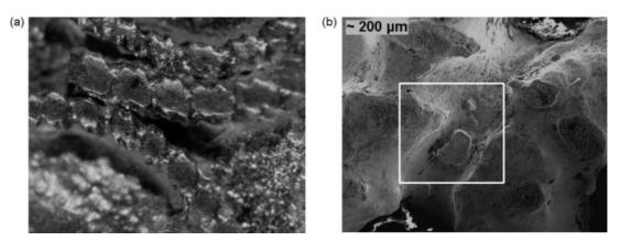
**Figure 1.** Wires joining by brazing on a gold plaque: (a) binocular image showing the joining region; (b) SEM SE image of the grain structure corresponding to the joining alloy with a filler pellet (source: M.F. Guerra, C2RMF).
