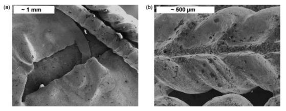
Figure 7. SEM SE details of the Etruscan finger ring: (a) the *repoussé* plaque rip; (b) modern drawn wires held on to the bezel by a huge amount of solder (source: M.F. Guerra, C2RMF).
