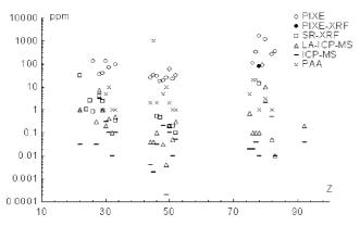
**Figure 5.** Detection limits of trace elements in gold alloys for the particular described analytical developments: filtered PIXE and PIXE-XRF, SR-XRF, PAA and ICP-MS in liquid and LA modes.
