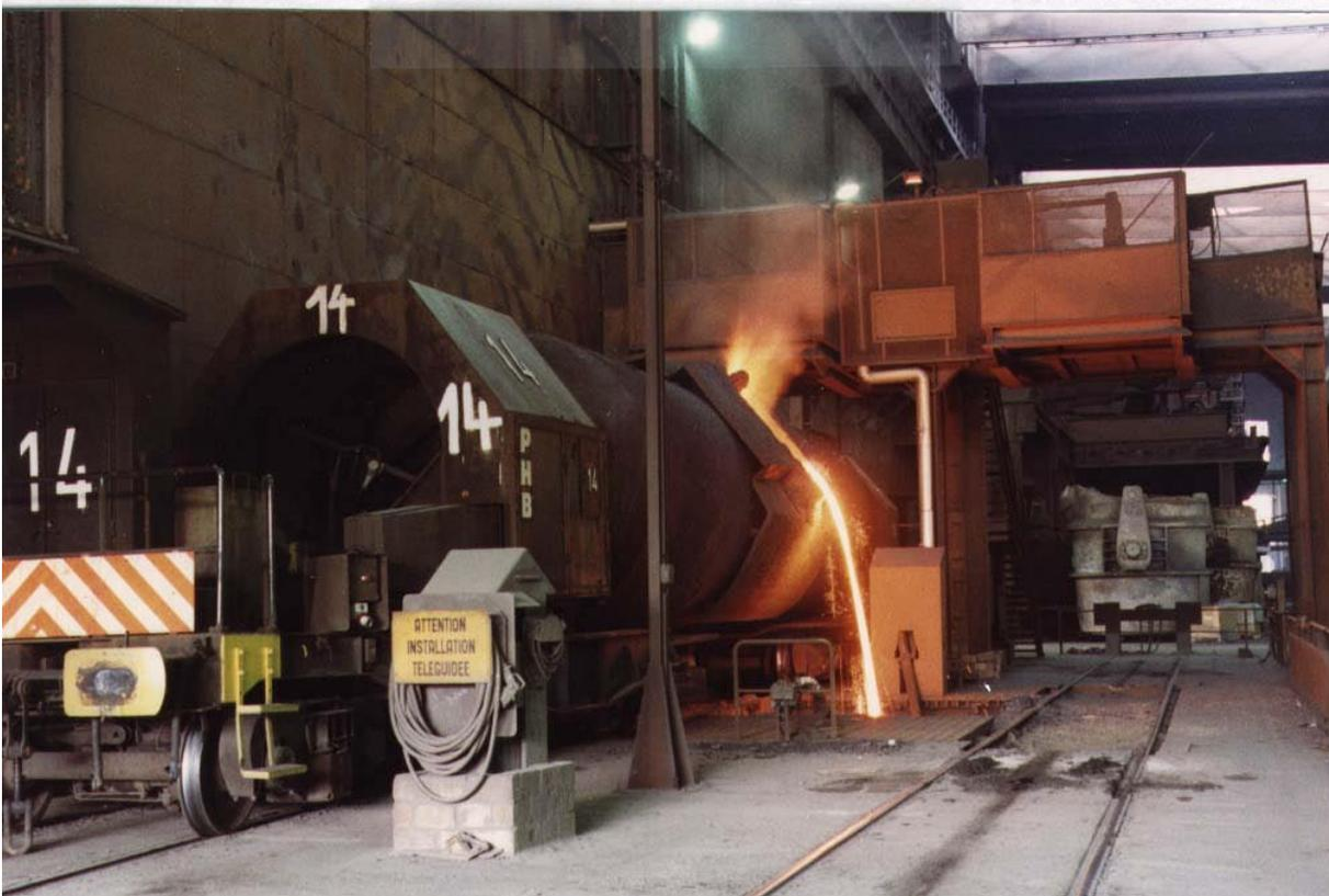
Figure 8.21: Reladling of hot metal from torpedo ladle to charging ladle with and without dust/fume suppression with inert gas (CO<sub>2</sub>) [UNEP, 1997]
