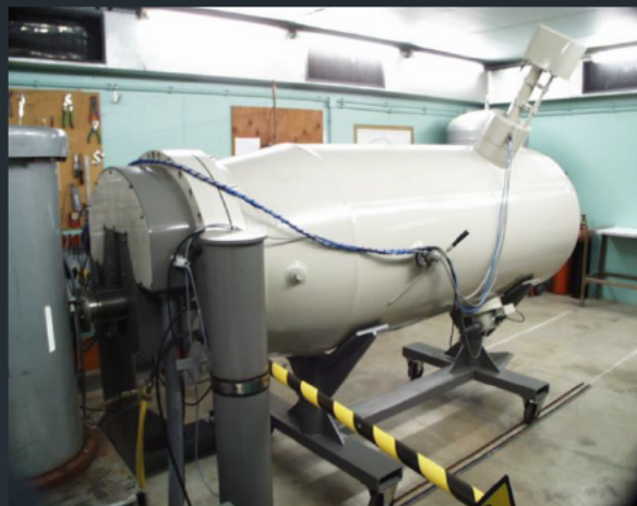
2.5 MV Van de Graaff accelerator at Campus Tecnológico e Nuclear, CTN/IST in Portugal.
