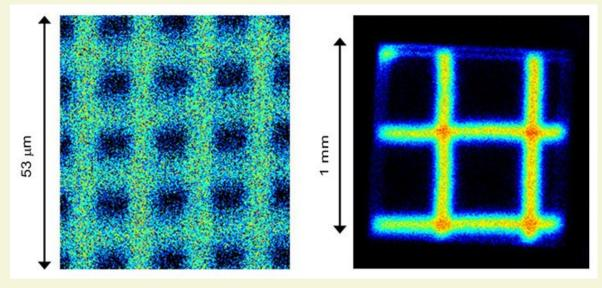
experimental conditions (proton beams of 2 MeV energy and 1 nA current). For the former, the spatial resolution is  $2x3 \ \mu m^2$  while for the latter external conditions the best spatial resolution is  $60x60 \ \mu m^2$  when working under helium rich atmosphere.
