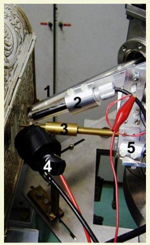
Figure 3. External beam set-up: 1. X ray detector; 2. mini-camera; 3. exit nozzle with a 100 nm thick  $Si_3N_4$  window; 4. particle detector with He flux; 5. Positioning lasers.
