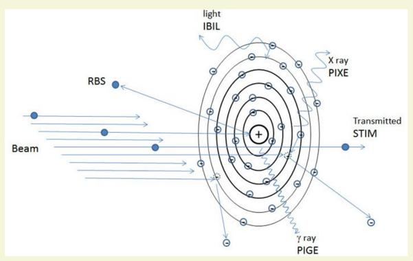
Figure 1. Scheme of interactions between ion beam particles and sample atoms with the corresponding IBA techniques.
