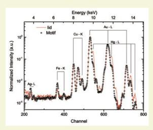
Figure 8. Normalized PIXE spectra from inside the cup (red) and an external gilt motif (black) of the ciborium (CMAG 1180 Collection).
