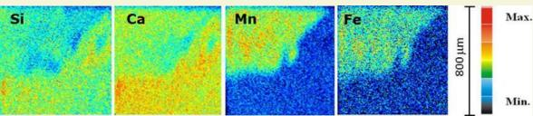
Figure 6. Elemental distribution of Si, Ca and Mn. On the corroded areas there is a higher concentration of Mn and Fe.
