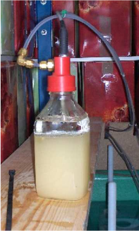
FIG. 2: a science C_2ClF_5 SDD during installation; the bottle is a squared 10 \times 10 \text{ cm}^2 base, 12 cm tall Schott glass containing \sim 900 \text{ ml} of freon+gel covered by a 6 cm glycerin layer. The cap contains the microphone and feedthroughs for the pressure (horizontal) and microphone (vertical) electronics.
