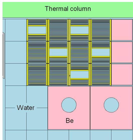
**Figure 1. Typical HEU core configuration, with 7 standard and 5 control assemblies.**
