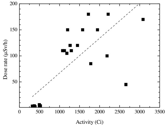
**Figure 3. Measured gamma dose rate at contact with the transfer cask, as function of the total assembly activity.**
