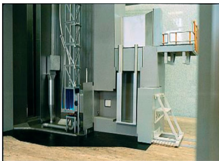
Figure 1 Schematic drawing (a) and picture of model (b) of the large sample neutron activation analysis facility in the thermal column of the Hoger Onderwijs Reactor in Delft.
