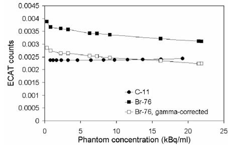
Figure 2 – HR+ 3D counts per second per voxel after decay, dead time and positron abundance correction. From [1].
