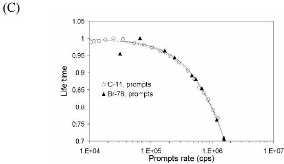
Figure 3 – Total dead time (A) and singles (B) and prompts (C) life times for  $^{11}\text{C}$  and  $^{76}\text{Br}$ , the singles life time with and without multiplication with a factor  $1+\delta$  to account for rejected photons.
