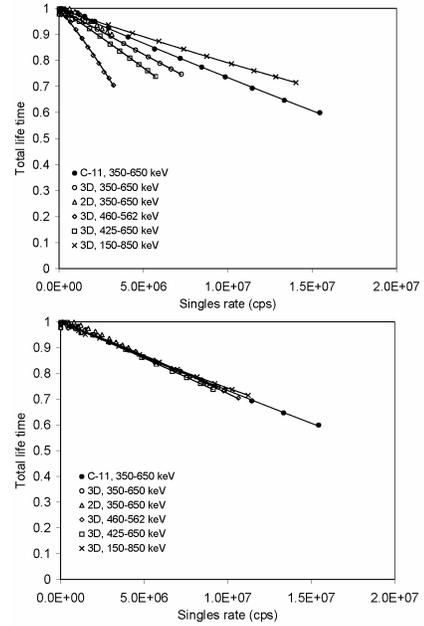
Figure 4 – Total life times versus singles rates of  $^{124}\text{I}$  for a number of different energy windows without (top) and with (bottom) consideration of rejected singles by multiplication of the singles rate with a factor  $1+\delta$ .
