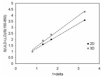
Figure 5 – Ratio of  $^{124}\text{I}$  singles rate in each energy window to that in the 150-850 keV window, compared to singles correction factor  $1+\delta$ .
